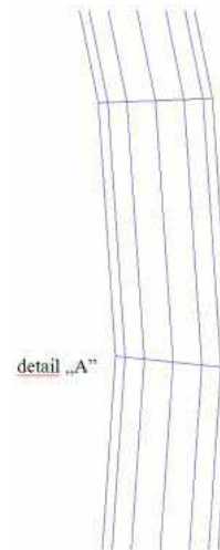
Figure 5: Elements through the thickness of the wall
